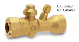
The **Type PZKP-BV** ball valve with forged brass body construction, integrated ZoomLock PUSH connections, and an access fitting, has full size ports to allow for unrestricted flow on all sizes. All PZKP-BV ball valves are bi-directional and may be installed in any position.
